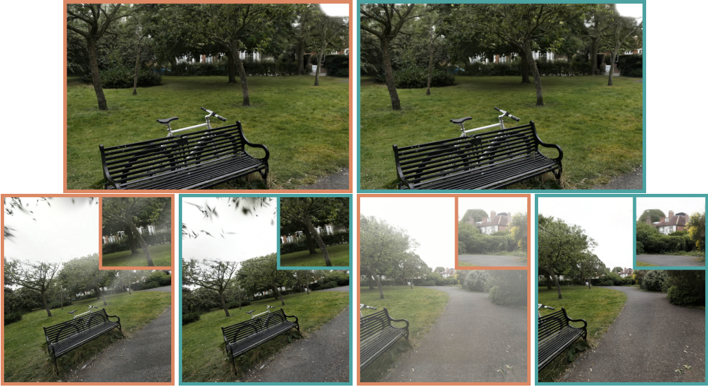
Fig. 2. Normal FOV (top) and VR (bottom) views of Mini-Splatting [Fang and Wang 2024] and ours . Increasing the field-of-view reveals shortcomings of current methods in VR applications: large Gaussians when projected with the local affine approximation can cause cloud-like artifacts and elongated Gaussians ( i.e. , “god rays”). VRsplat eliminates the artifacts while meeting the performance demands of smooth VR experiences.
