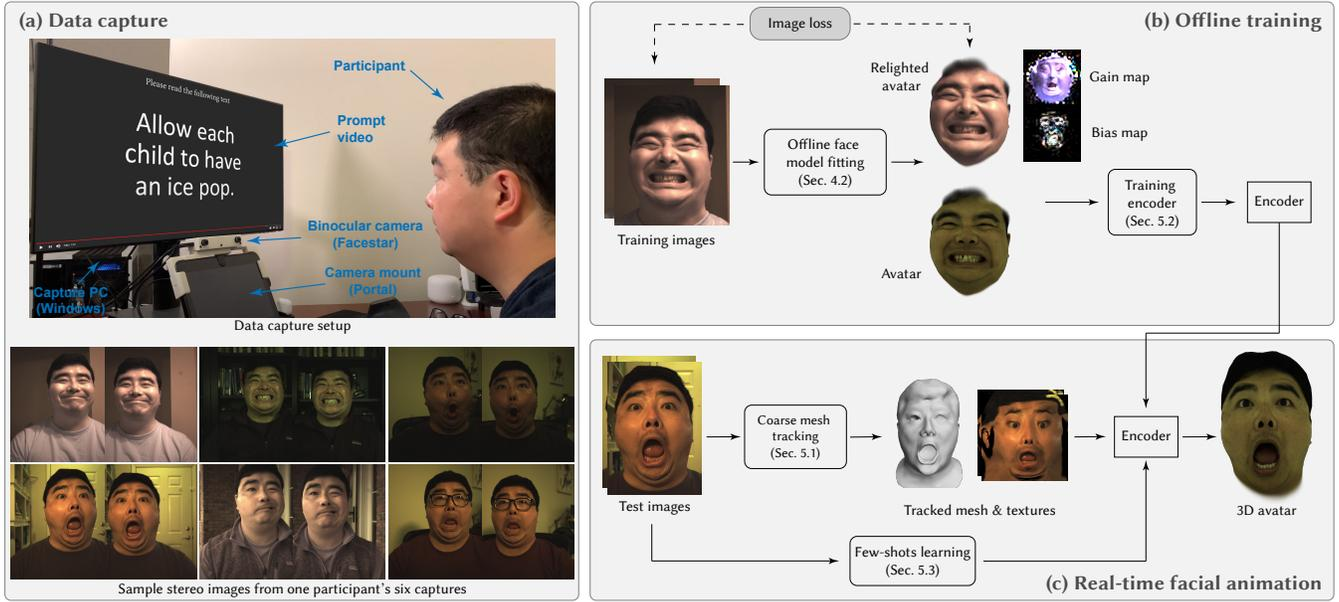
Fig. 2. Overview of our method. We use the binocular camera Facestar to capture user’s facial performance in different environments (a). We then fit the DAM to the captured images, to get the groundtruth face parameters for each frame, which are used to train the encoder (b). The pre-trained encoder then can be used to drive the avatar animation in real-time (c).
