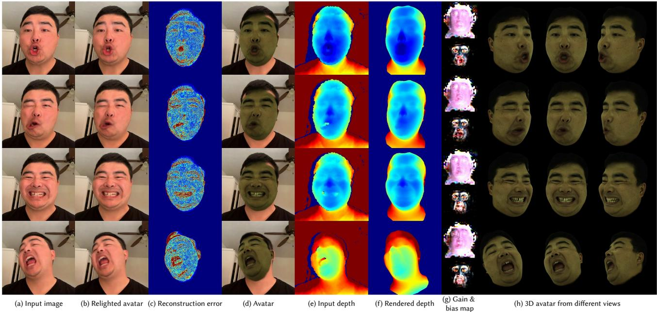
Fig. 8. Off-line face model fitting on iPhoneXS data. With input image (a) and depth (f) from iPhoneXS, our algorithm estimates accurate face parameters to animate the avatar with the closely matching facial expression and motion (b, d, g).
