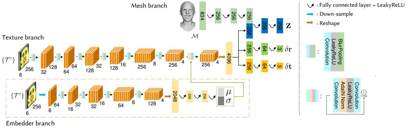
Fig. 7. The network architecture of encoder. We have three branches in encoder. From top to bottom: mesh branch, texture branch and embedder branch. The output of embedder branch,  $\mu$  and  $\sigma$  are used as parameters for the adaptive instance normalization (AdaIN Norm) in the last convolution layer in texture branch.
