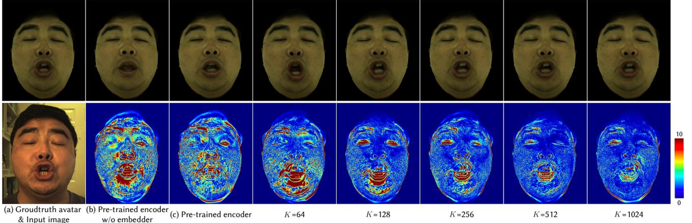
Fig. 11. Ablation study on few-shots adaptation. Directly apply the pre-trained encoder to the test video will fail in tracking accurate facial motions. With more frames from test video in adapting the encoder will help to get more accurate avatars, but brings more computation time. In our experiments, we find  $K = 256$  can already give satisfying results.
