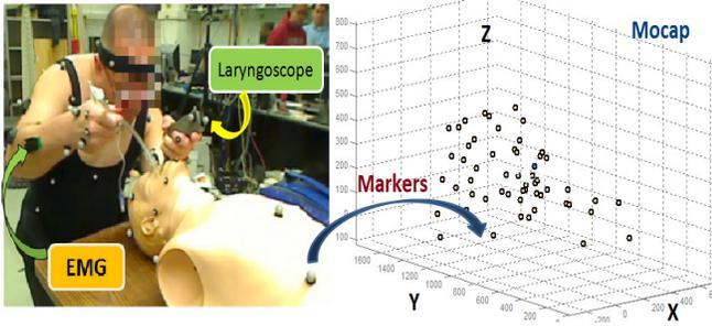
**Fig. 1.** This figure demonstrates the experimental setup. The providers are fitted with reflective markers (white spheres) as well as EMG/accelerometer sensors while they performed intubation on a dummy. The 3D marker trajectories of all the markers were tracked during the entire procedure (one frame is shown on the right).
