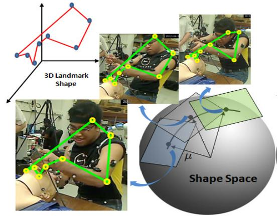
**Fig. 2.** This figure demonstrates how we represent the temporal movement patterns of left arm/head w.r.t the dummy's mouth as a sequence of deforming 3D landmark shapes.
