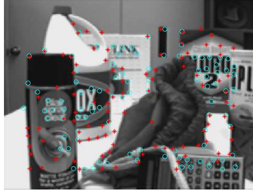
Fig. 8 Selected feature points based on two different criteria. Cyan circles: 100 points selected using Shi & Tomasi criterion. Red stars: 100 points selected using our criterion. Selected feature points of each method are at least 10 pixels apart.
