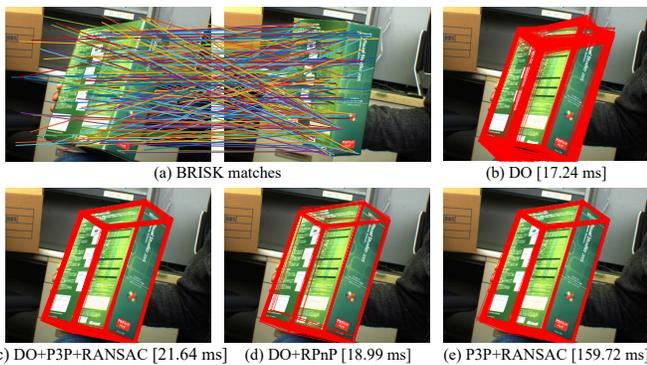
Figure 7. Results for camera pose estimation on real image. (a) Feature matches. Left and right images contain 2D points and projection of 3D points, *resp.* (b-d) Projected shape with average time over 100 trials.
