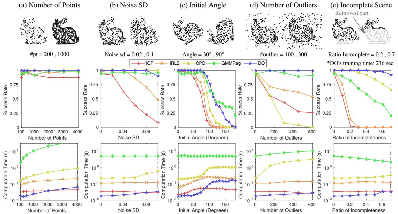
Figure 3. Results of 3D registration with synthetic data under different perturbations. (Top) Examples of scene points with different perturbations. (Middle) Success rate. (Bottom) Computation time.
