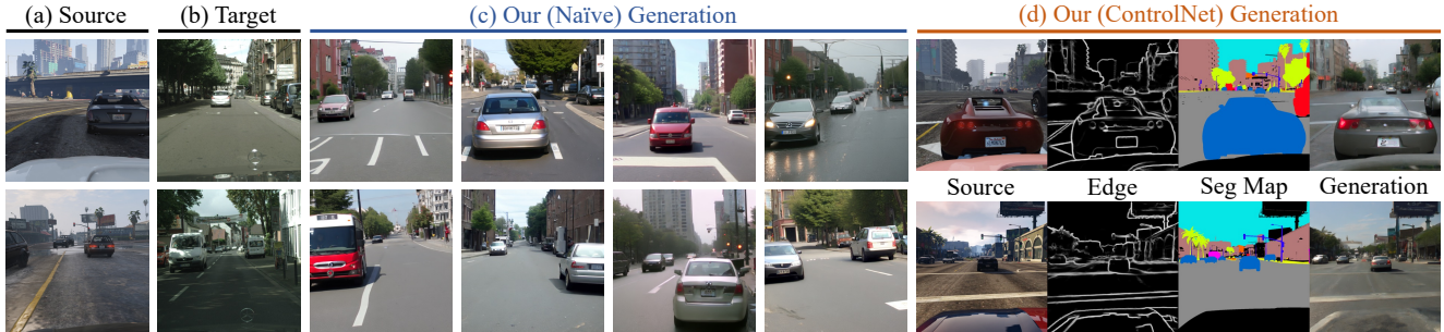
Figure 5. Examples of synthetic self-driving data generated from (a) GTA5 source images into (b) Cityscapes target domain. (c) shows the synthetic data generated from our pipeline without any improvement tricks. We also demonstrated the generation with scene structure preserved by ControlNet (conditioned on canny edges and source segmentation ground truth) in (d). The synthetic data are then used in unsupervised domain adaptation methods to adapt models across domains.
